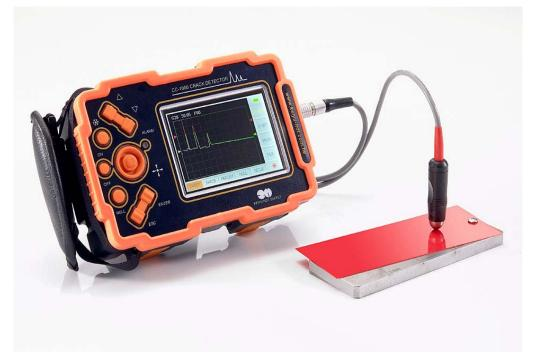
CC-1000 SURFACE CRACK INDICATOR IS AN MAGNETIC FIELD TECHNIQUE FOR DETECTING FATIGUE CRACK IN FREEOUS WELD OR ROW MATERIAL. THIS INSTRUMENT GREATLY REDUCED THE COST AND TIME THAN ALTERNATIVE
