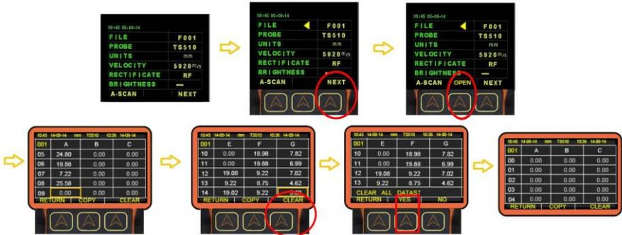
By pressing MODE key **M** to enter configure manual, press function key **A** under NEXT, then press function key **A** under CLEAR. The display will ask “Yes” or “No”, Press function key **A** under “Yes” to clean all of data. The file F001 will empty and waiting entry new data.
