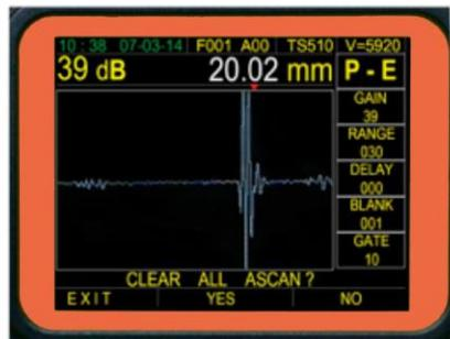
By pressing green arrow key under “SAVE” to recall A-scan files, then press **C** the display will show “CLEAR ALL ASCAN?”, press green arrow key under YES, all A-scan files will be cleared out.
