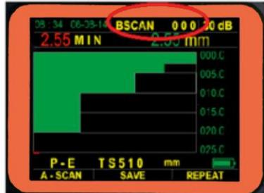
By pressing **M** enter to manual, then press green arrow key under “OPEN” to open B-SCAN files.
