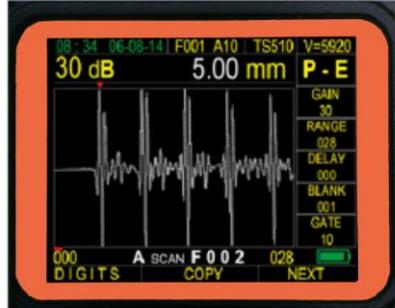
For example put probe on step block 10 mm thick, after display stable to remove the probe from test block, then press green arrow
