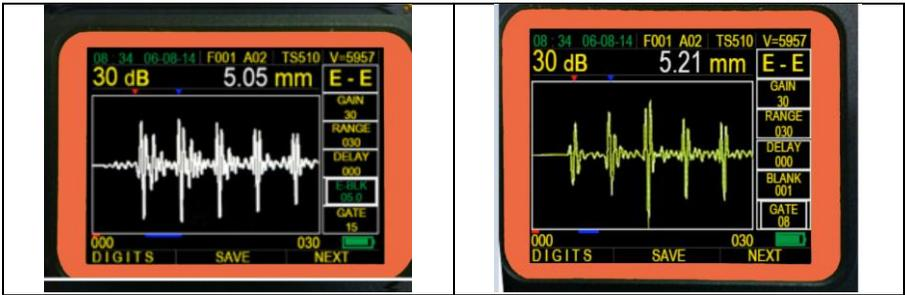
We use blank red bar del.. noise echo from first echo. Use blue bar E-black del. the noise echo between first and second echo.
